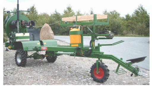
The SuperPak netmachine is a self-transportable netmachine that can be towed by at car with trailer connetion.
